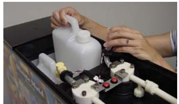
Load new package and replace check valve
