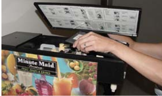
Remove Top Cover and Splash Tray over Pump Assemblies
