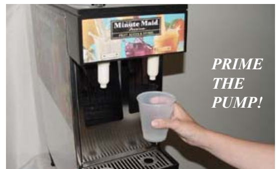
Prime pump by dispensing approximately eight ounces of product from the nozzle or until there are no air bubbles present in the concentrate tube
