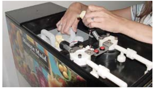
Remove Check Valve from empty package and remove package
