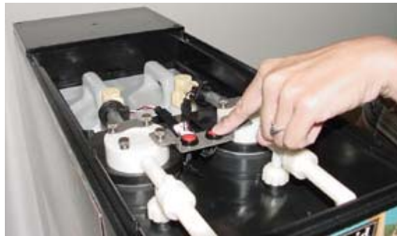
Press red reset button next to the pump for the product just loaded. The Product Out lights will turn off. Replace Splash Tray and Top Cover
