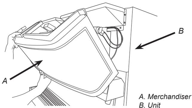
5. Unplug the low ice indicator cable inside the merchandiser on the left side of the unit, before removing the merchandiser.
