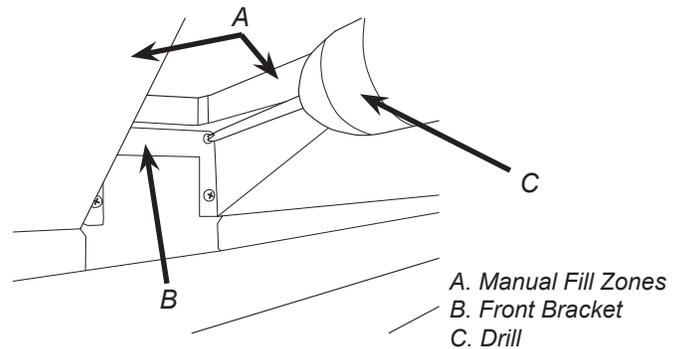
8. Once the bracket is removed, reinstall the four (4) bracket screws.
