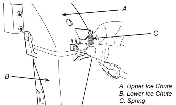
4. Remove the existing lower ice chute by carefully spreading apart the bracket arms connected to the upper ice chute.
