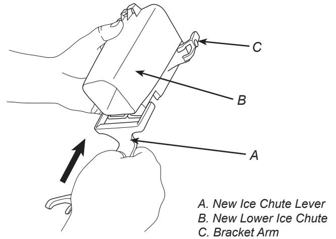
7. Attach the new lower ice chute assembly, installed in the previous step, to the existing upper ice chute by aligning the front of the lower ice chute to the upper ice chute then gently rotate the back of the lower chute until it locks in place.
