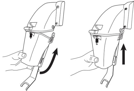
8. Connect the spring, removed in Step 5, to the newly installed lower ice chute assembly and the existing upper ice chute.
