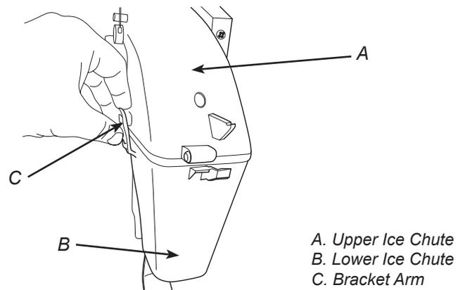
5. Remove the spring, detached in Step 3, from the lower ice chute.
