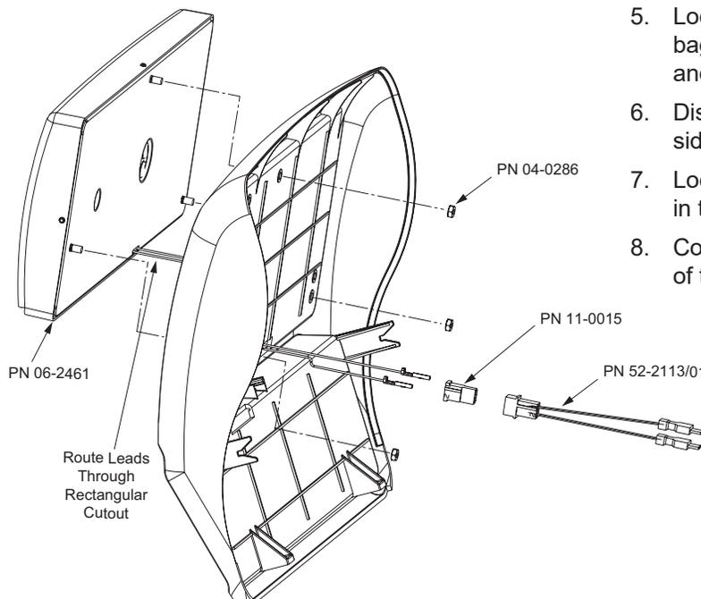
9. Reconnect the leads from the key switch to the piggy-back connections on the Lead Extension Assembly.
